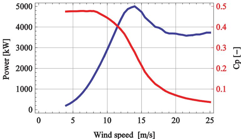
Figure 3: 5 MW DeepWind baseline design power curve (blue) and  $C_p$  (red)
