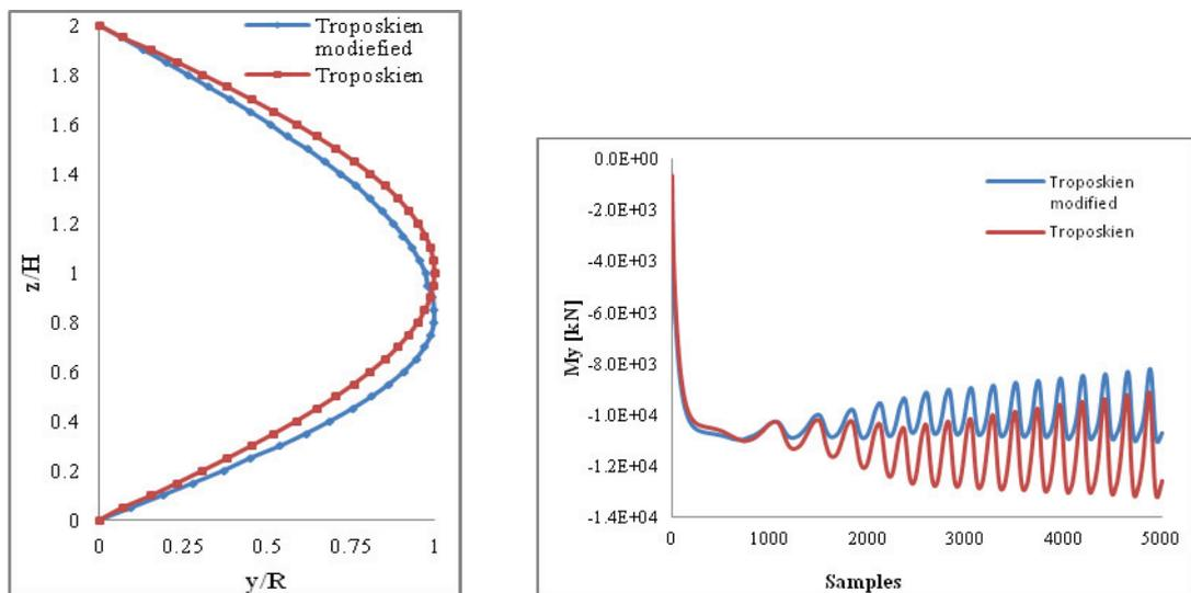
Figure 4: Left: Two different blade shapes according to two different operational conditions. Right: Loads corresponding to the two different rotor shapes [3].
