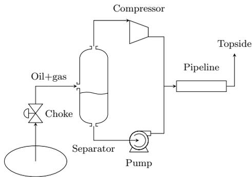
Fig. 1. Subsea gas compression station
