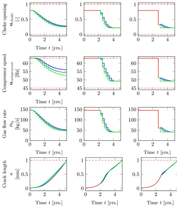
Fig. 6. Three snapshots of the closed-loop solution at  $t = 0$ ,  $t = 2$  and  $t = 2.8$  yrs. The blue, turquoise and green scenarios are for the low, expected and high realizations of the stochastic parameter  $c_{Paris}$ , respectively. The maintenance horizon is fixed at 5 years.
