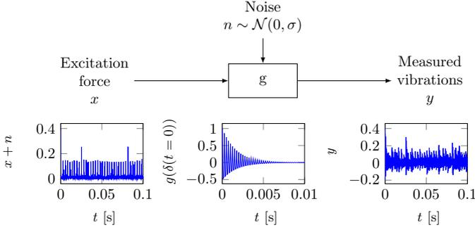
Fig. 3. Signal path from excitation force  $x$  to measured vibrations  $y$ , via impulse response model  $g$ .
