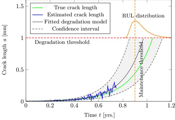
Fig. 4. Illustration of estimated degradation model based on "measurements" of the crack length (which themselves are estimated from vibrational data)
