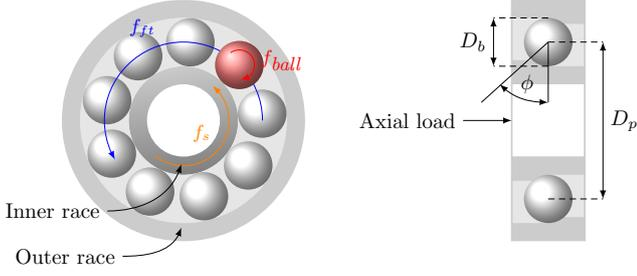
Fig. 2. Illustration of a ball bearing
