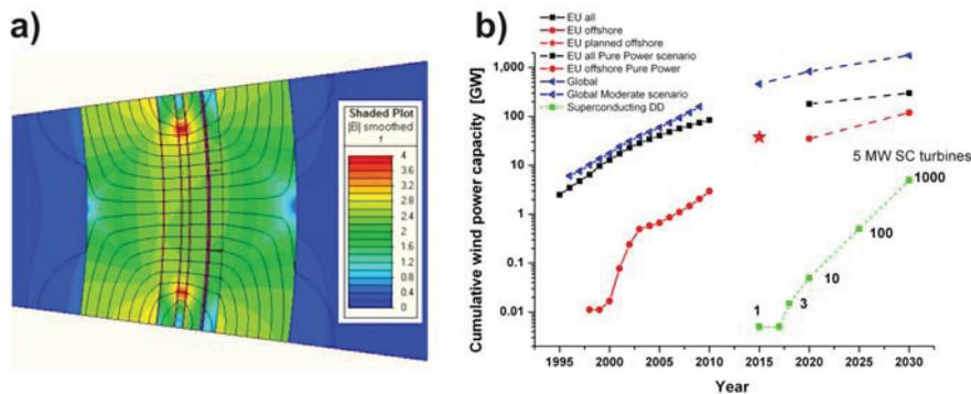
Fig. 5. a) Magnetic flux density of a 24 pole generator. From left: rotor steel, cryostat, superconducting windings and support, cryostat, air gap, armature windings and stator steel. b) Roadmap of introduction of superconducting wind turbines in the European off-shore market. Reproduced from [7, 8].
