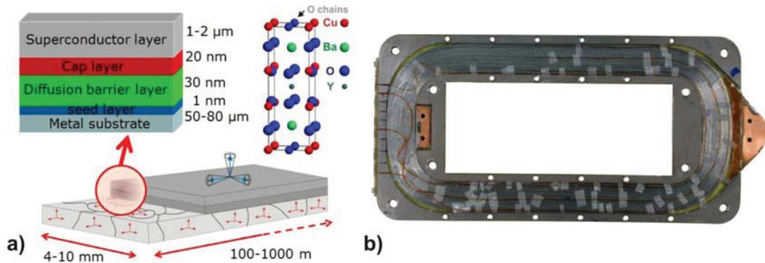
Fig. 2. a) Architecture of coated conductor based on bi-axially aligned  $\text{YBa}_2\text{Cu}_3\text{O}_{6+x}$  high temperature superconductor deposited on textured buffer layers and a metal substrate. Inset: Crystal structure of YBCO. Reproduced from [8]. b) Example of racetrack coil wound from 30 m or 70 m of coated conductor tape from American Superconductor and Superpower, respectively. Reproduced from [7].
