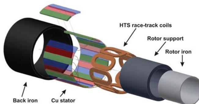
Fig. 1. The main components of a superconducting multi-pole generator. Reproduced from [5].
