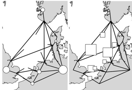
Fig. 2. Base case - NSOG for year 2030 including both existing and planned interconnections. Offshore wind connections are also included with higher transfer capacity than the installed offshore wind capacity, in order to narrow the scope to a pure interconnection analysis. Relative peak load (left plot; circles) and relative offshore wind capacity (right plot; squares).
