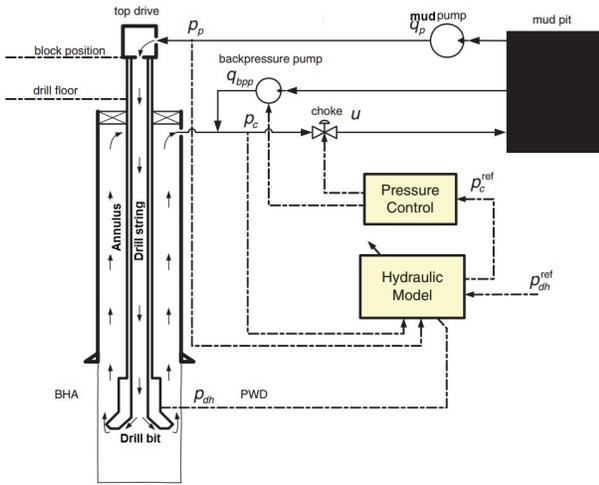
Fig. 1: Schematic of an automated MPD system (Statoil).
