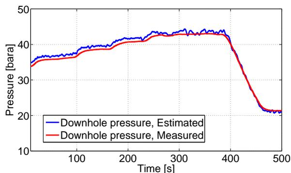
Fig. 5: Estimated and measured downhole pressure.
