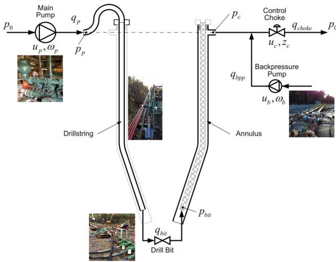
Fig. 2: Schematics of the flow-loop.
