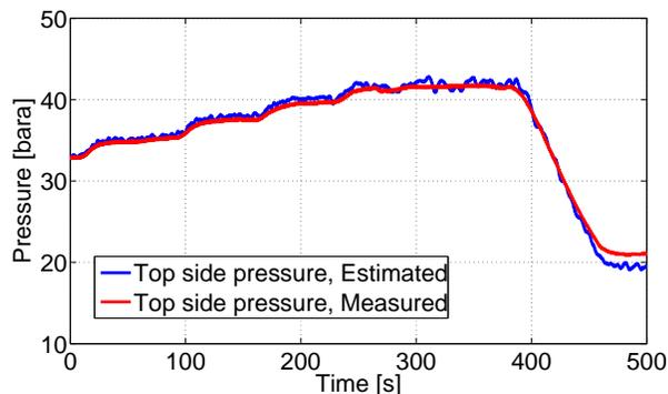
Fig. 7: Estimated and measured topside pressure.
