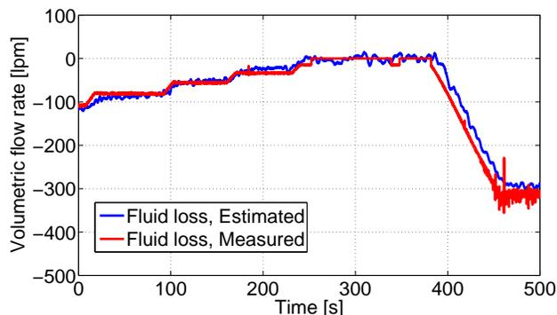
Fig. 6: Estimated and measured fluid loss at the bottom of the well.
