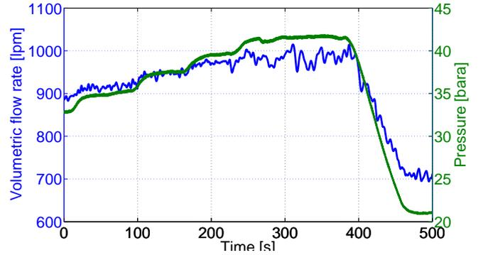
Fig. 3: Measured topside flow rate (coriolis meter) and pressure.
