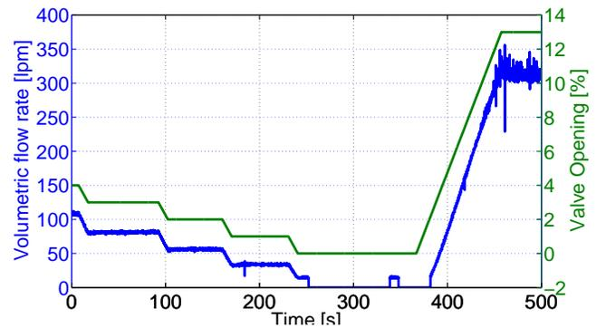
Fig. 4: Downhole exit valve opening and volumetric flow rate response.
