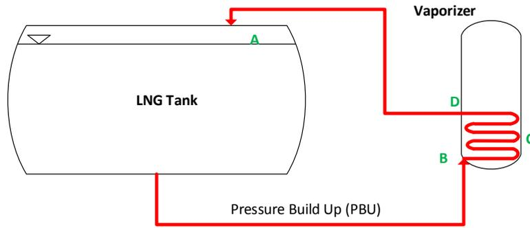
Fig. 2. Different Piping Section of the Pressure Build Up (PBU) Unit
