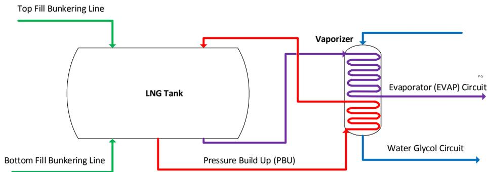
Fig. 1. Schematic of the LNG tank and Vaporizer system on KV Bergen and MF Korsfjord
