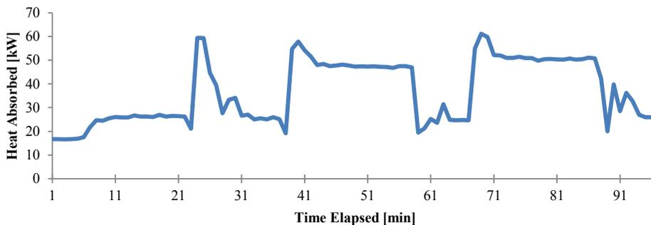
Fig. 4. Heat Absorbed by the Evaporator while MF Korsfjord Transits
