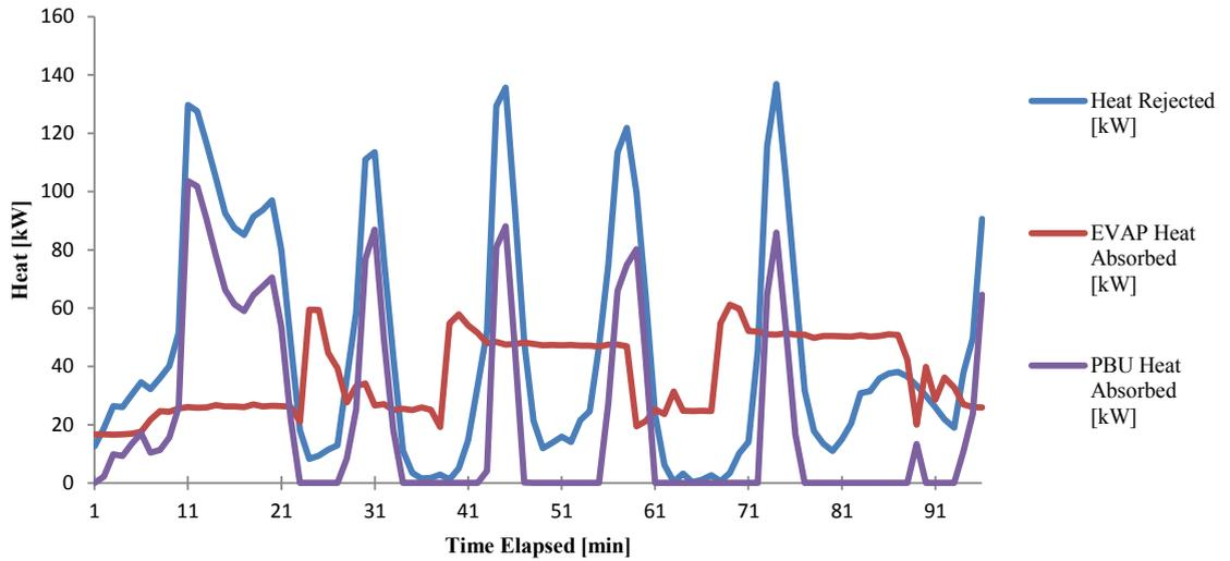
Fig. 5. Heat Exchange between the Water Glycol (Heat Rejected), EVAP and PBU (Heat Absorbed) in the Vaporizer based on measurements onboard MF Korsfjord
