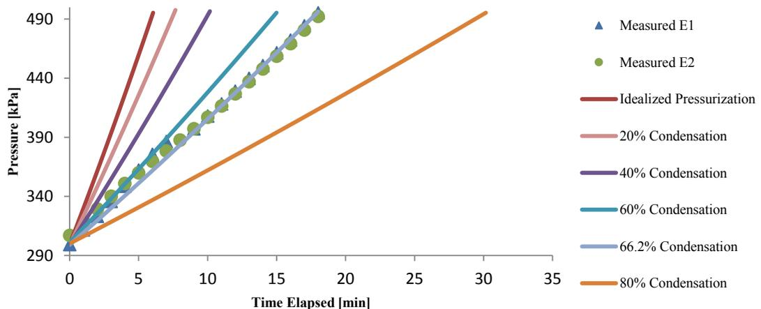
Fig. 7. LNG Tank Pressurization Time with Vapor Condensation
