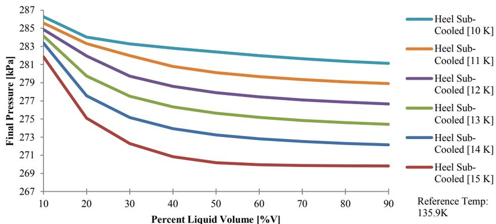
Fig. 3. Final Tank Pressure After Complete Liquid and Vapor Mixing Given Different Initial Liquid Temperatures
