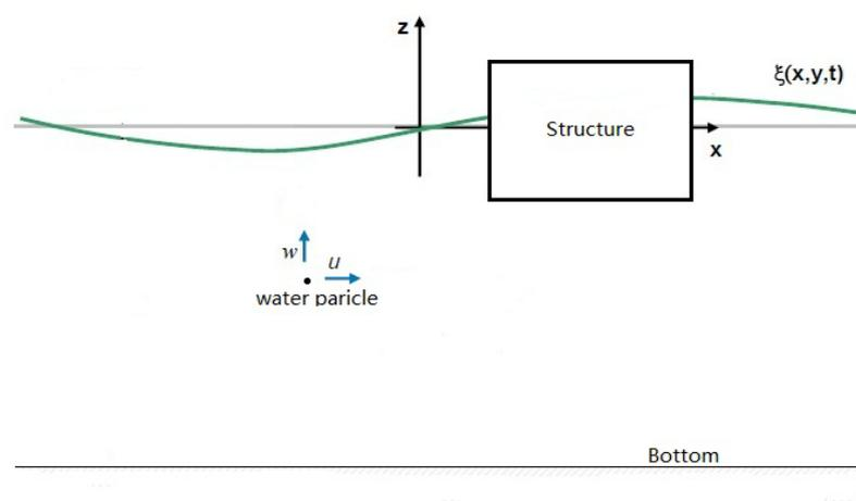
Figure 2.1 Offshore structure in regular wave
