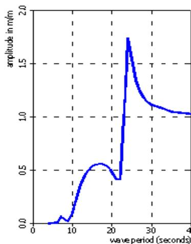
Fig 5.1 Transfer function for heave motion of aimed structure
