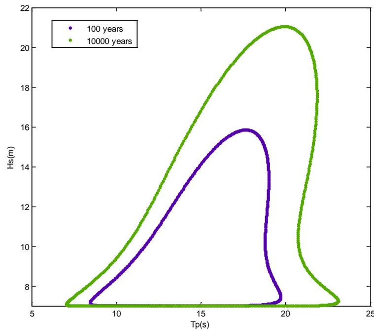
Figure 7.2 Contour lines using storm peak characteristics
