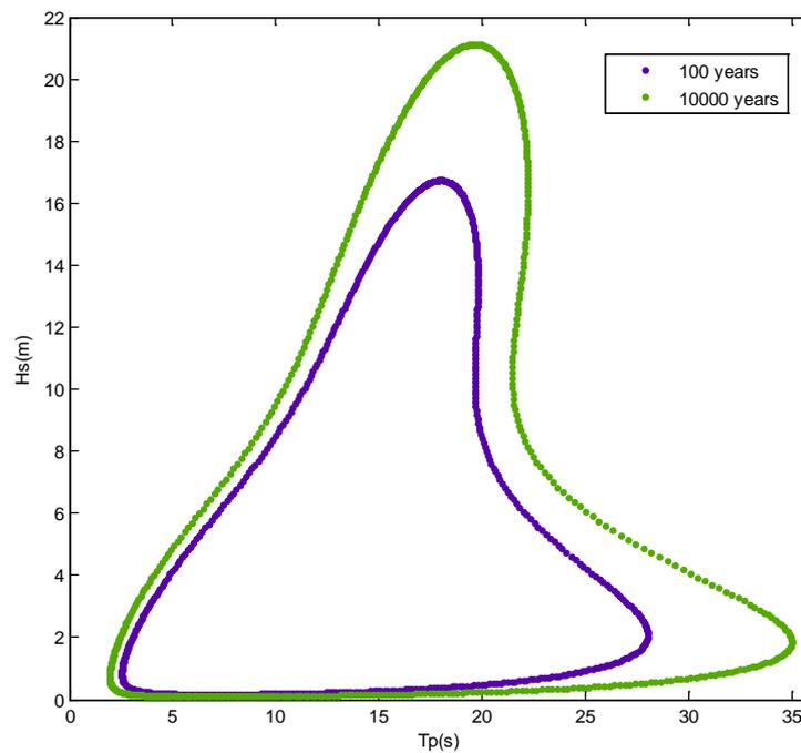
Figure 7.1 Contour lines using all sea states characteristics
