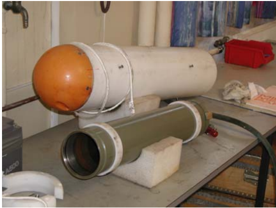
Figure 5: Electronic pressure case and its protection
