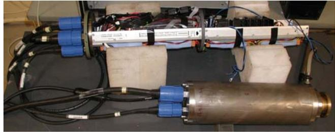
**Figure 6:** Electronics and Motor pressure case
