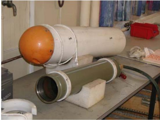
**Figure 5:** Electronic pressure case and its protection
