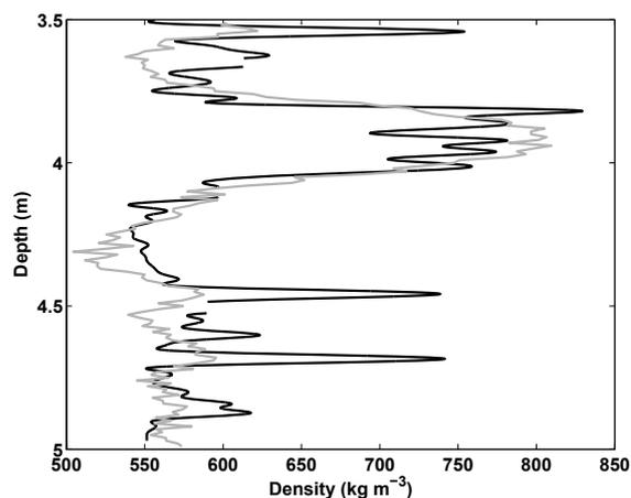
**Fig. 4.** A 'pseudo-density' profile, derived from the COS profile and a simple linear transformation, is shown in black with the NP-density data in grey. Note that while not giving a true physically based measurement of density, the COS-derived pseudo-density profile clearly captures the details of the ice layers.
