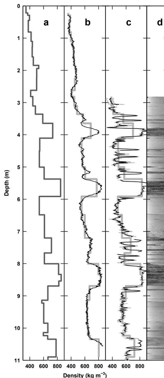
**Fig. 2.** Density data (black) and data averaged over core sections (grey) to facilitate comparison: (a) gravimetric density data; (b) NP data; (c) DEP data (thin grey lines depict four runs at 0, 90, 180 and 270° rotation, and the black line depicts the mean); and (d) imagery of the core on a black background with side illumination, the basis of the COS shown in Figure 3.
