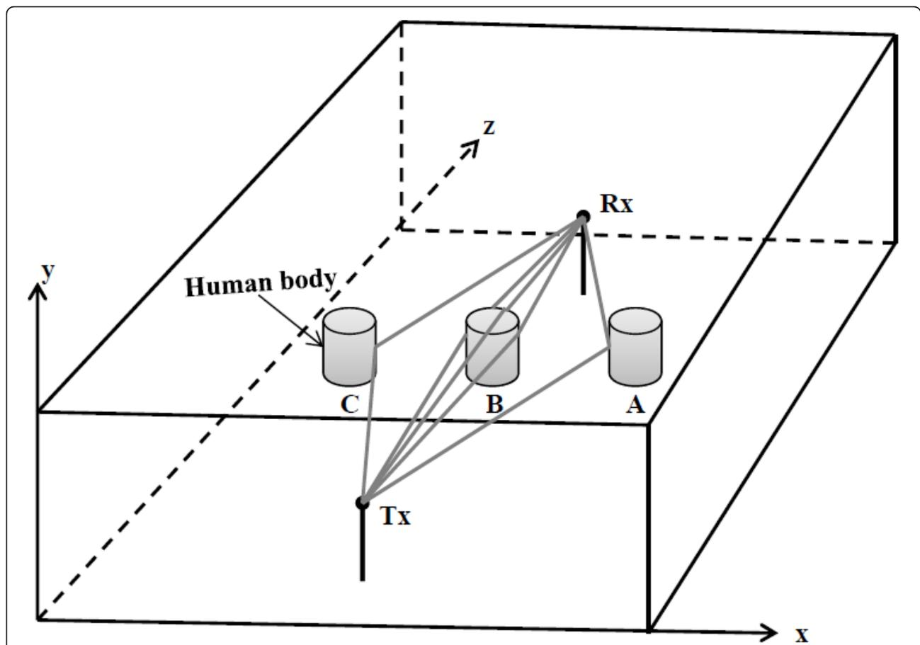
**Figure 1** Propagation scenario for signal shadowing by moving human body in indoor environment. The indoor propagation environment is defined by orthonormal vectors  $x$ ,  $y$  and  $z$  of a rectangular coordinate system. The person is walking in the direction ABC or CBA. The LOS path is crossed at position B. Tx and Rx are the transmitting and receiving antennas, respectively.
