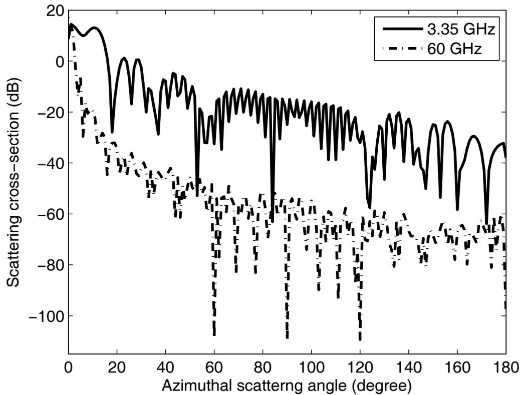
**Figure 5** Scattering cross-section of a dielectric cylinder representing a human body at 3.35 GHz and 60 GHz. The simulation parameters are given in Table 1.
