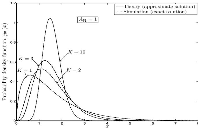
Fig. 2. The PDF  $p_{\Xi}(x)$  of the received signal envelope at the output of the EG combiner  $\Xi(t)$  for a different number of diversity branches  $K$ .
