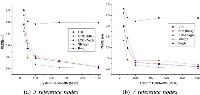
Fig. 4. Performance comparison in OLOS channel.
