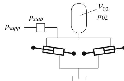
**Fig. 6** Pendulum bar stabilizing system circuit
