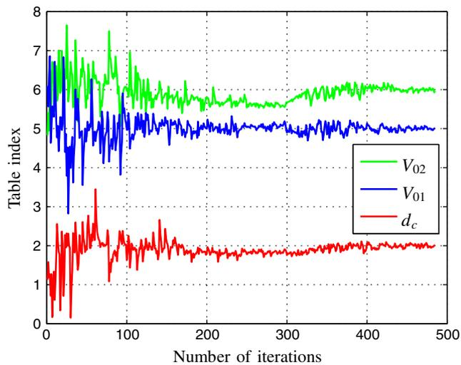
**Fig. 13** Development of the three discrete design variables with decreasing  $\epsilon$
