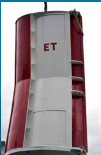
Figure 4: Trawl doors with hatches that can be opened/closed to adjust performance while fishing.
