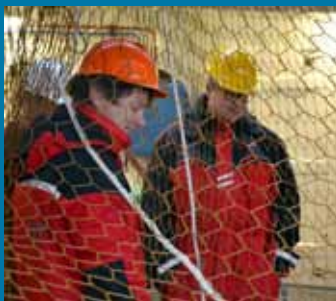
Figure 3: Hexagonal meshes shaped as a brick wall can become the future trawl net.
