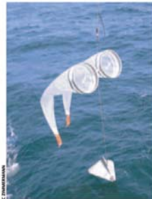
A Bongo plankton net, used for the sampling of herring larvae in the Greifswalder Bodden since 1977
